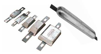
Despite all these goals, some problems may arise when zinc anodes are used in fresh water and especially in high-temperature applications. Since 1939 it is known that common zinc alloys tends to fail at temperature above 60°C. In these situations, anode suffers passivation and may give rise to the phenomenon of polarity reversal, a dangerous condition in which zinc and steel reverse their natural polarity and steel becomes anodic to zinc, corroding itself to protect the anode.
